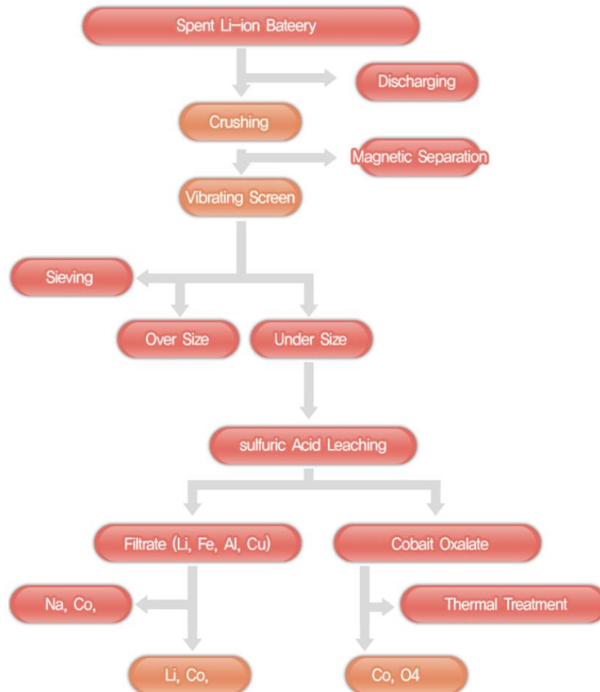
Figure 14: Flowchart of Li-ion battery recycling process published by Kobar [68].
