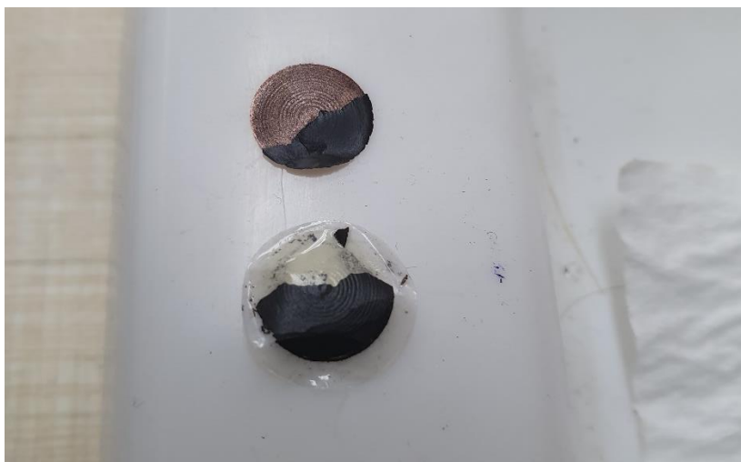
Figure 18: Image of the Gen-1 electrodes after 50 cycles at 100% DoD.
