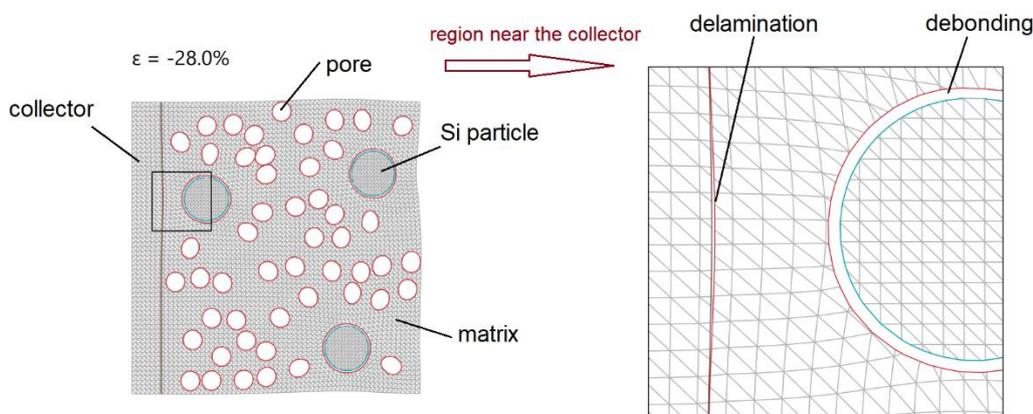
Prediction of shrinkage of the Si particles embedded into a porous matrix in a periodic computational domain.
